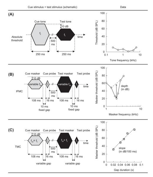
**Figure 1.** First column: schematic representation of the test stimuli in measures of (A) absolute threshold (250-ms tone), (B) iso-forward masking contour (IFMC), and (C) temporal masking curve (TMC) measure. Second column: examples of the data obtained in the absolute threshold, IFMC (with  $f_t = 2$  kHz) and TMC measure for a listener with good hearing, plus illustration of depth and slope measure for IFMC and TMC respectively.
